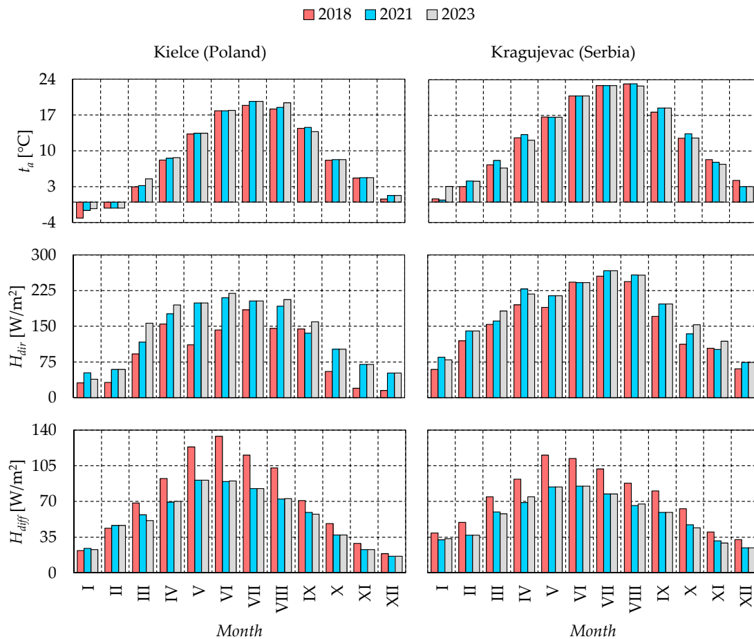
Figure 5. Monthly weather files for Kielce (Poland—continental climate zone) and Kragujevac (Serbia—moderate continental climate zone) during 2018, 2021 and 2023.
