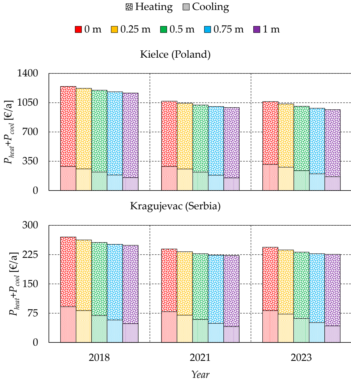
Figure 12. Annual monetary expenses for heating and cooling in the analyzed small advanced single-family house models.
