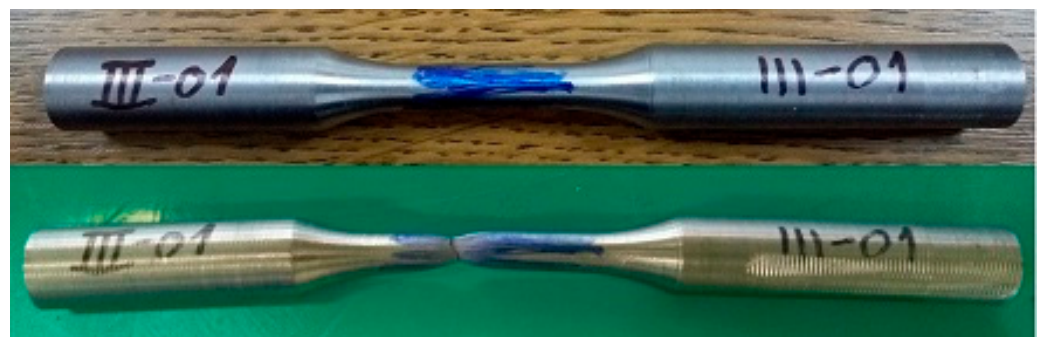
Figure 7. Failure modes for cyclic tension–compression test specimens.
