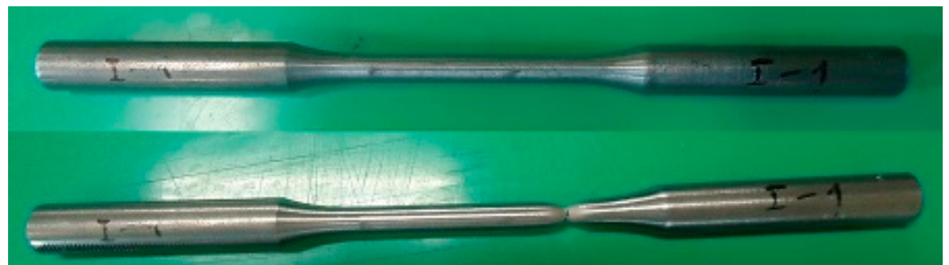
Figure 6. Failure modes for monotonic tension test specimens.
