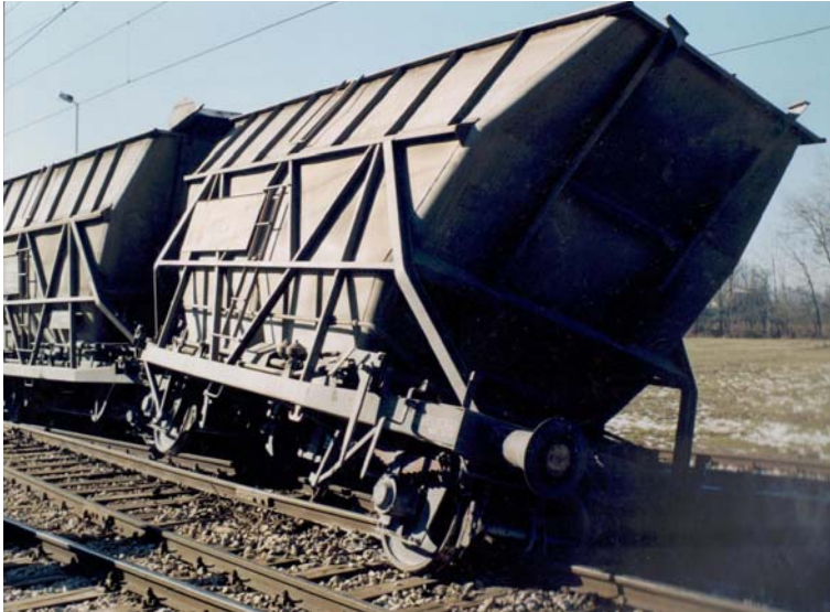
Fig. 1. The derailment caused by the failure of the suspension system
