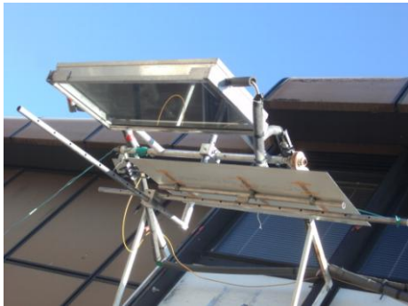
Figure - Experimental installation of the double exposure (left) and conventional solar collector (right)
