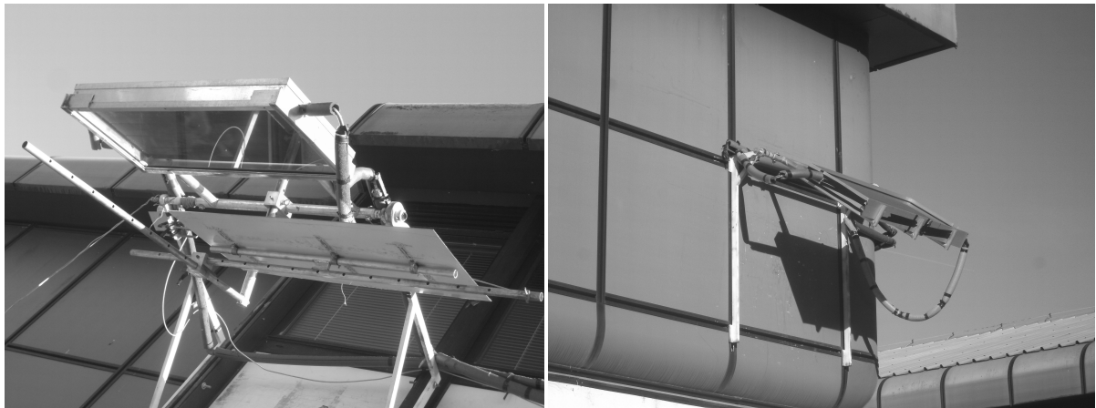
Fig. 1. Experimental installation of the double exposure (left) and conventional solar collector (right)
