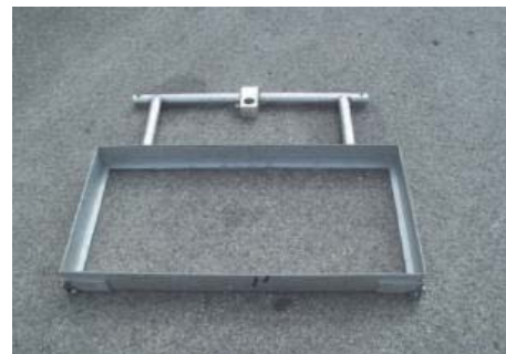
Fig. 2 The supporting construction of the CRS (left) : 1-cantilevered bracket, 2-axle with dividing head and 3-collector bracket, and the collector bracket (right)
