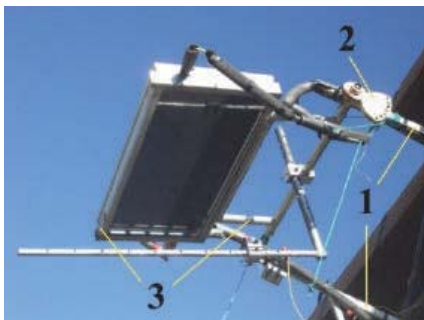
Fig. 2 The supporting construction of the CRS (left) : 1-cantilevered bracket, 2-axle with dividing head and 3-collector bracket, and the collector bracket (right)
