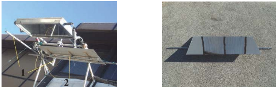
Fig. 3 The construction for reflector movement (left): 1-rectangular frame and 2-reflector frame, and the reflector (right)
