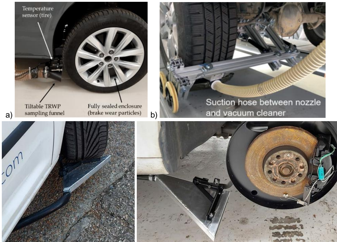
Figure 14 Variants of devices on vehicles for drawing in and measuring particles produced by tire wear in case of road tests, a) first variant, b) second variant, c) third variant [36, 37, 38]
