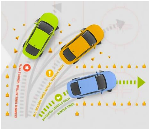
Figure 5 The influence of the type of tire on the cornering of the vehicle [11]
