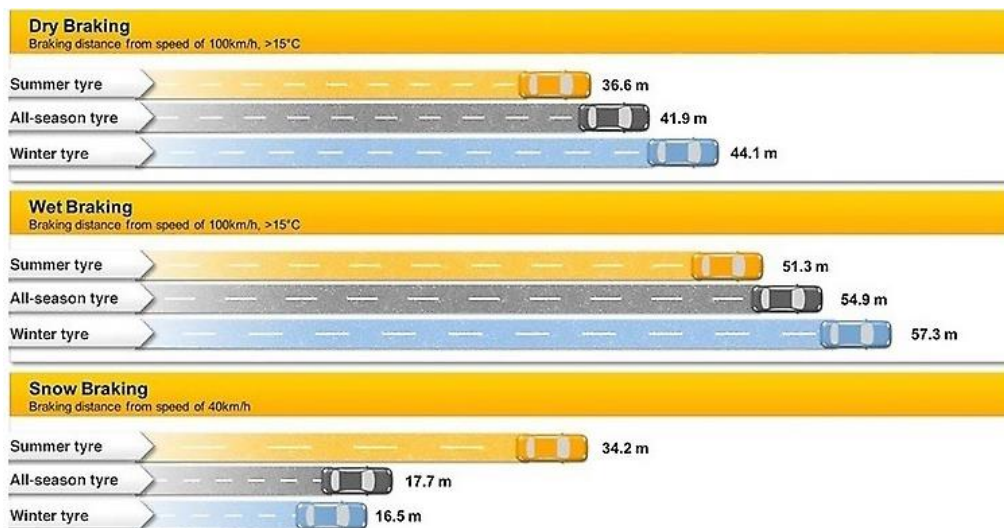
Figure 3 Dependence of braking distance on tires and braking conditions [8]
