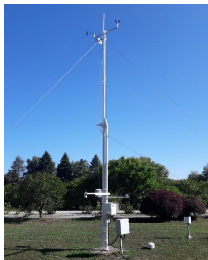
Figure 1. MicroStep-MIS weather station scheme and experimental setup.
