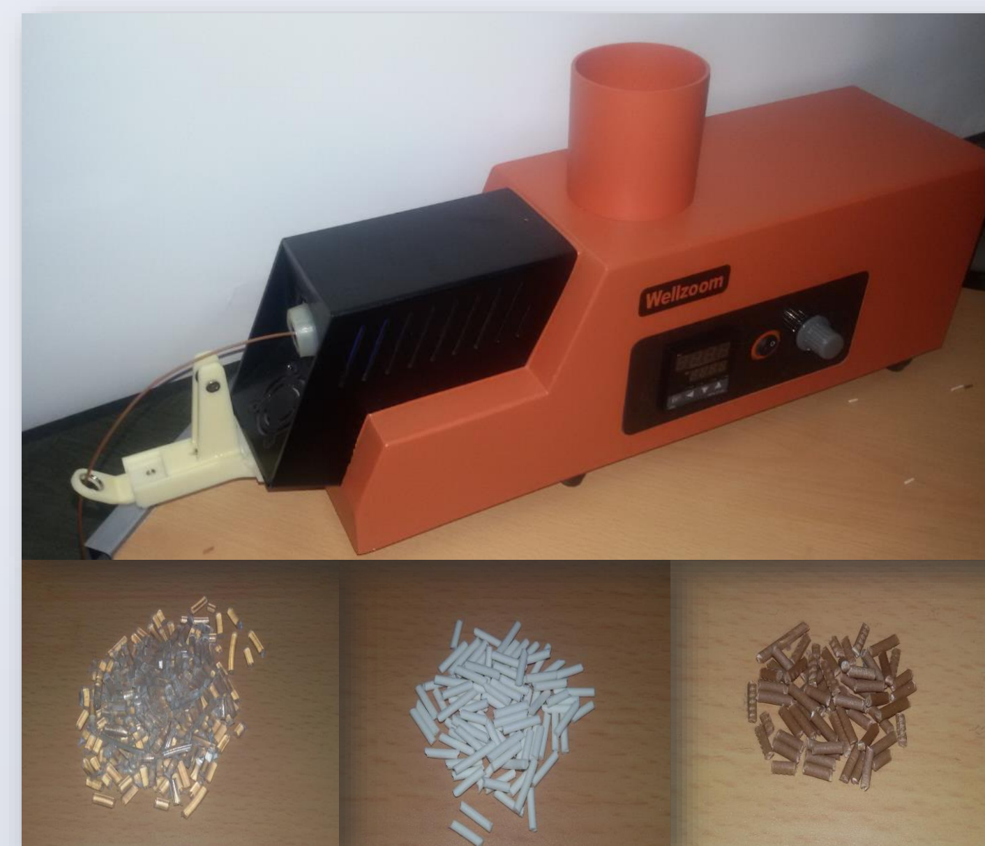
Figure 1. Desktop filament extruder and three different materials, Center for Information Technology (CIT), Faculty of Engineering, Kragujevac
