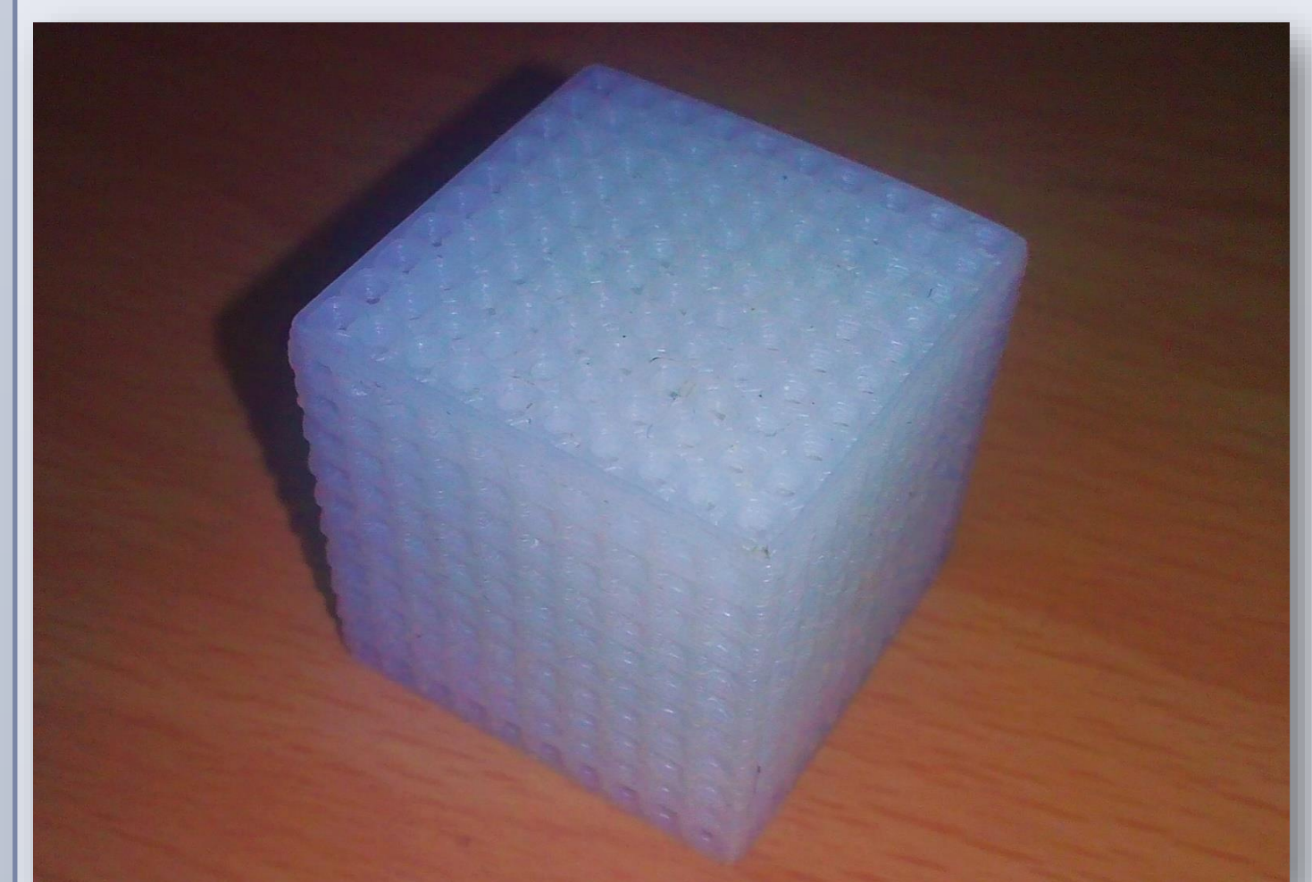
Figure 7. 3D printed scaffold for tissue engineering
