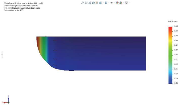
Fig. 7. Representation of the deformed state of the composite vessel
