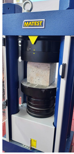
Fig. 1. Experimental investigation of concrete specimen in compression testing machine
