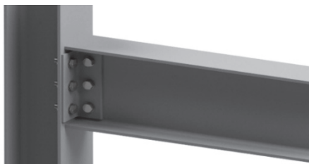
Fig. 2. Web cleat connection
