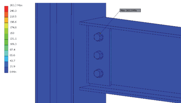
Fig. 8. Place of maximum contact pressure for FP
