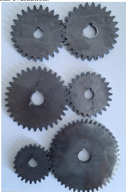
Fig. 2. Laser-cut produced spur gear pairs
