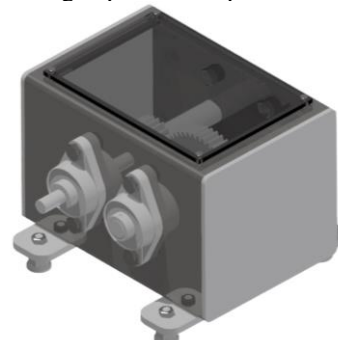
Fig. 9. 3D model of the dedicated gearbox module with a gear ratio of 1.42 – side view
