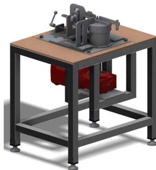
Figure 1. Pin on Disc Tribometer
