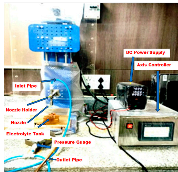
Figure 2. Experimental setup of ECJM at IIT Bombay.
