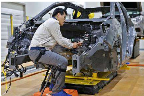
Fig. 2. Example of an exoskeleton that takes on the role of a "chair" [8]
