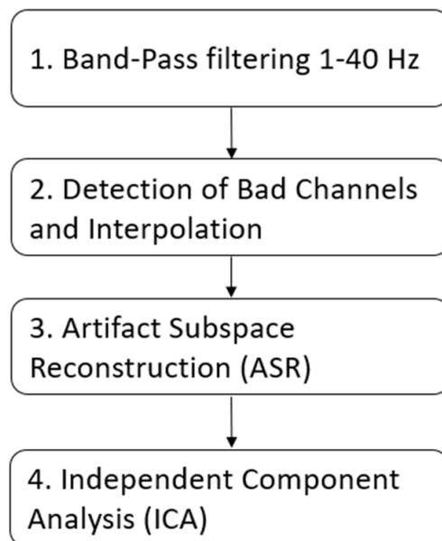
**Figure 6.** Flowchart of the EEG pre-processing phase.
