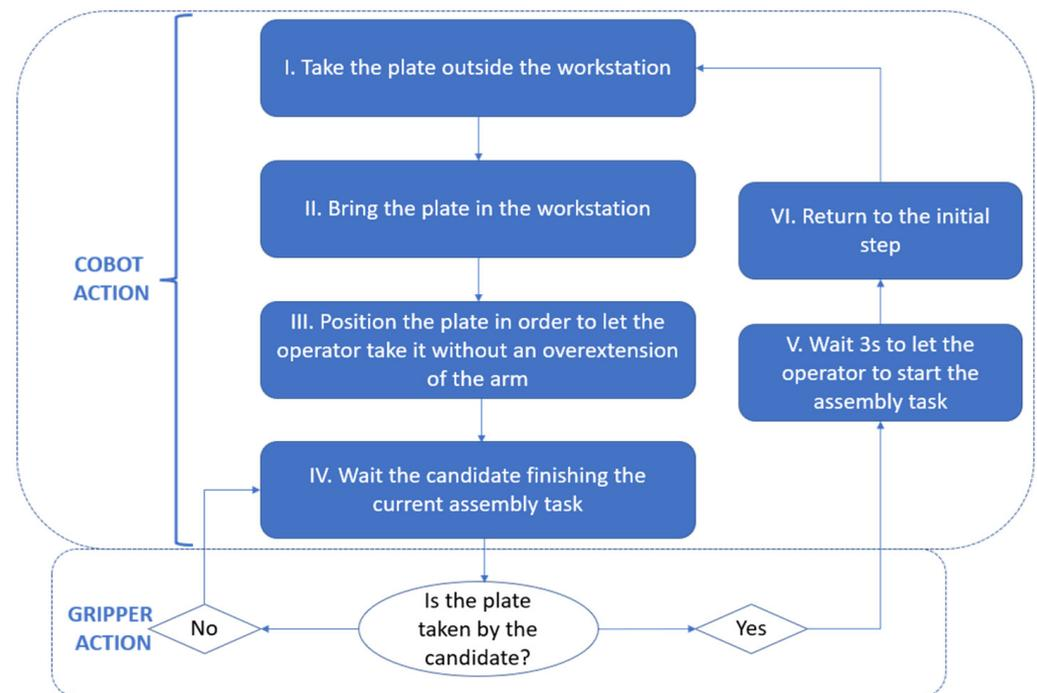
**Figure 4.** Sequential collaboration: cobot and gripper action logic.
