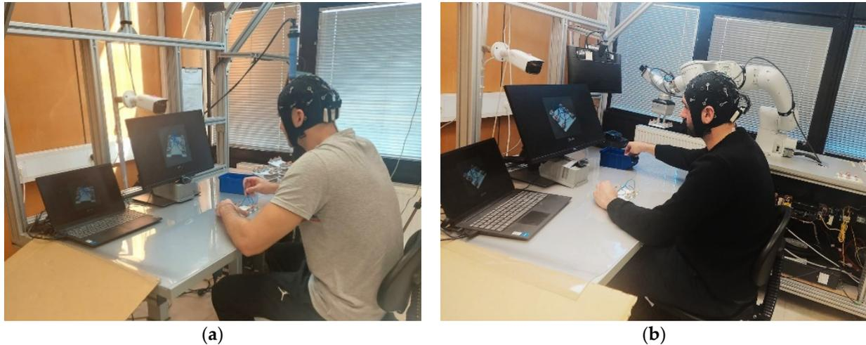
**Figure 2.** (a) Standard scenario (SS): the assembly task is performed by the participant without any external intervention in the workplace and (b) collaborative scenario (CS): the assembly task is performed by the participant interacting with the robot in the workplace.
