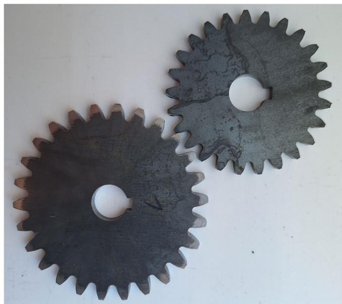
Figure 4. Unfinished and finished side of the laser-cut gears.
