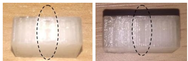
Figure 16. Worn PLA blocks under lubricated conditions
