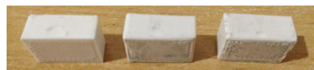
Figure 15. Worn ABS blocks under dry conditions
