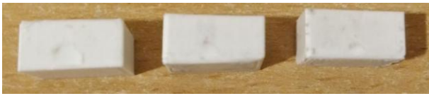
Figure 18. Worn ABS blocks under lubricated conditions
