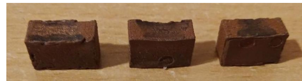
Figure 14. Worn PLA + copper blocks under dry conditions
