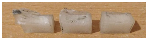
Figure 13. Worn PLA blocks under dry conditions
