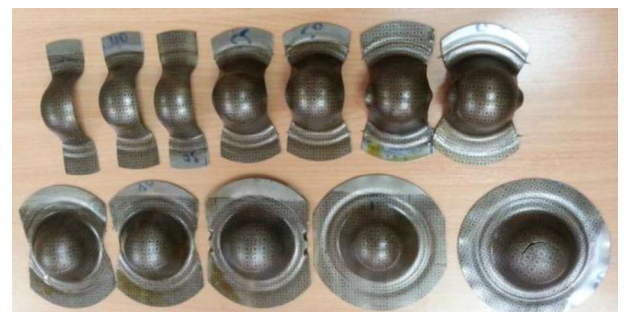
Fig. 1. Sheet metal samples made of DC04 material for FLD determination
