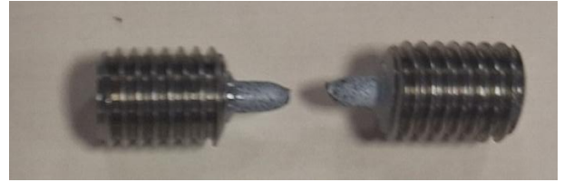
Fig. 5. Fractured S1100QL specimen; single neck centered in the gauge.
