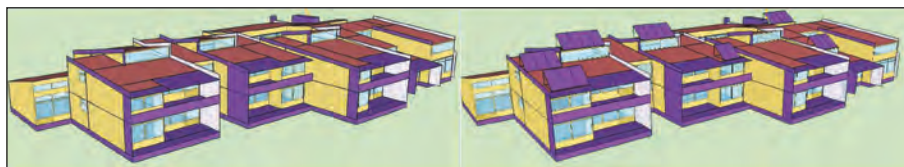
Figure 1. Isometric view of the building (left), isometric view of the building with 23 PVs installed (right)
