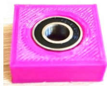
Fig. 6. Final appearance of the press-fitted bearing within the 3D-printed PET-G housing, illustrating proper alignment and seating of the component after assembly.
