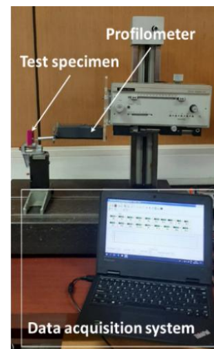
Fig. 5. Surface roughness testing on the profilometer.
