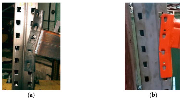
Figure 3. Experimental deformation of class A connection under single cantilever test in the following: (a) the panel zone of a steel rack connection (reprinted from Ref. [60]). (b) Column perforation and hooks (reprinted with permission from Ref. [61]. Copyright 2024, Elsevier).
