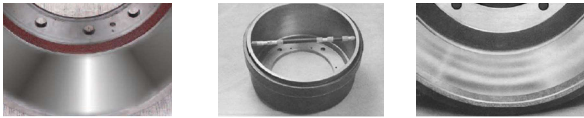
a) b) c) Figure 4. a) Polished drum, b) Drum deformation, c) Excessive wear Source: [6,7]
