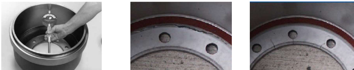
a) b) c) Figure 5. a) Oversized (worn) drum, b) Mounting ring cracking, c) Radial cracking of the bolt holes Source: [5,6]
