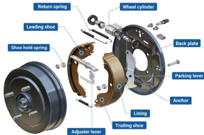
Figure 1. Components of the drum brake mechanism
