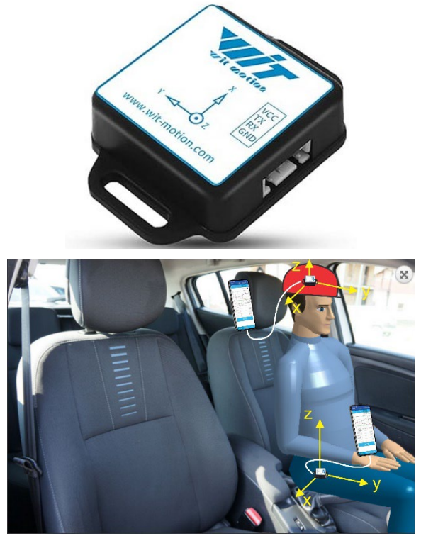
Fig. 1. Six-axis acceleration sensor (up); Schematic of the in-vehicle experiment setup (down)
