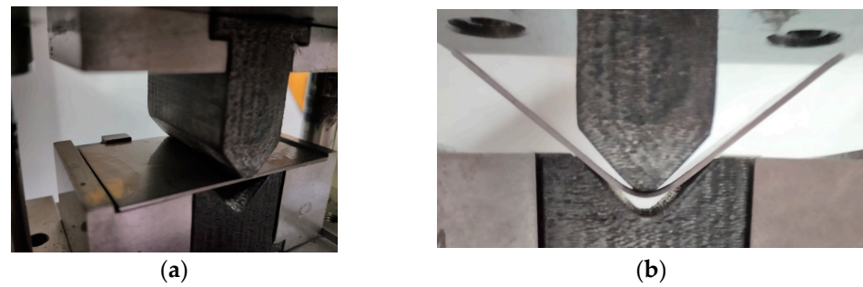
Figure 24. ABS tool mounted on the machine: (a) at the beginning and (b) during the air-bending process.
