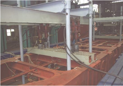
Fig. 8. Testing of static strength of flat wagon
