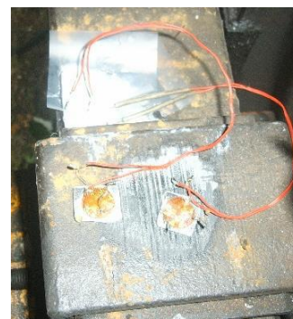
Fig. 13. Measurement of dynamic stresses of wagon's parabolic leaf spring
