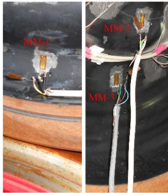
Fig. 14. Measurement of stresses at specific points on rail wheel
