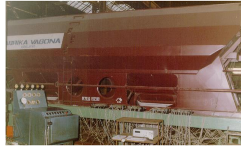
Fig. 9. Testing of static strength of closed freight wagon
