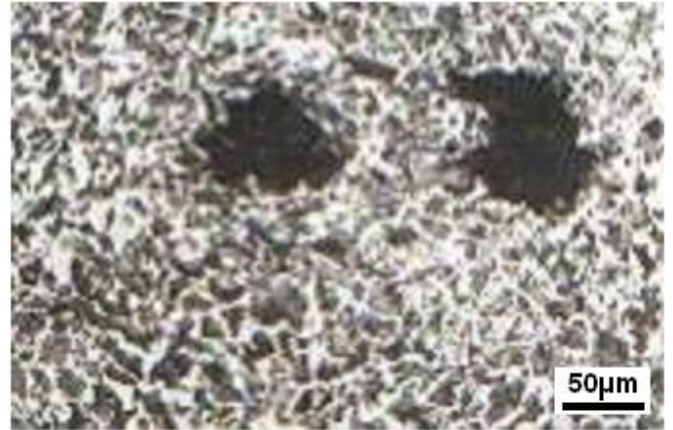
Fig. 13. The gas bubbles in the weld metal
