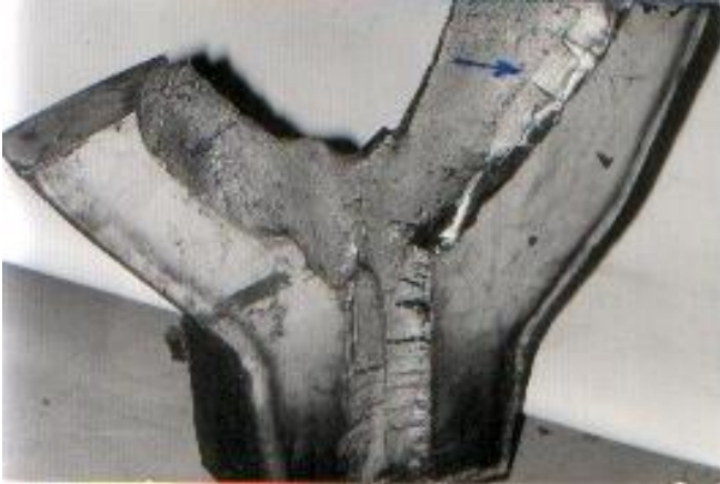
Fig. 10. The fracture surface of satellite carrier flange with indicated low-cycle fatigue (blue arrow)
