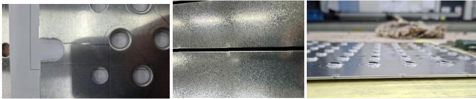
Fig. 5 Some of the defects that occur during punch pressing: punches extending beyond the sheet edge (left), poor cutting of parts (uneven edges) (middle), and skewed collars around punched holes (right)
