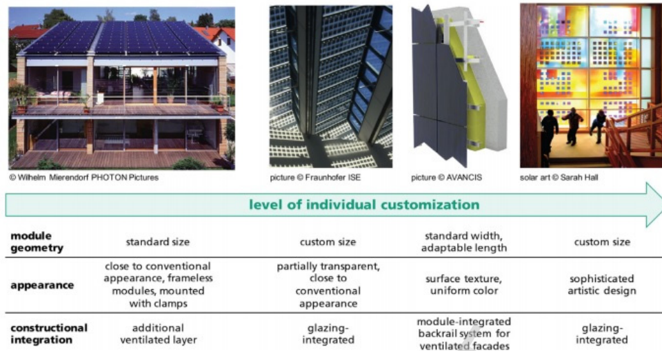
Figure 1: Overview of BIPV systems through examples [2]
