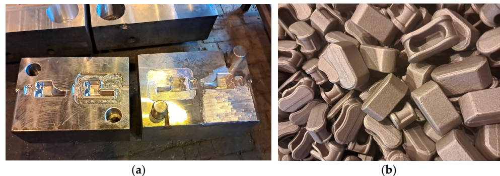
Figure 4. Specialized forging die (a) and finished forging (b).
