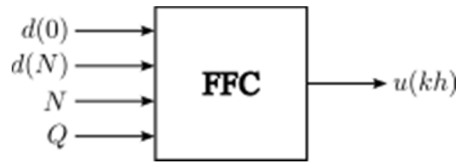
Figure 3: Feedforward controller (FFC)
