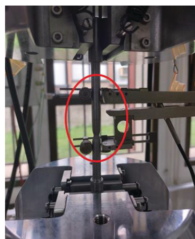
Fig. 2. Elongation measurement using extensometer
