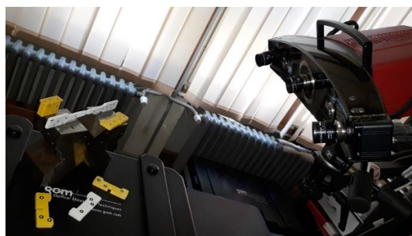
Fig. 1. GOM Atos optical measuring system measuring specimen tested for tension
