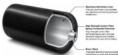
Figure 1 Design of a Type 3 Composite Cylinder (AA6061 aluminium liner with carbon fibre/epoxy overwrap)
