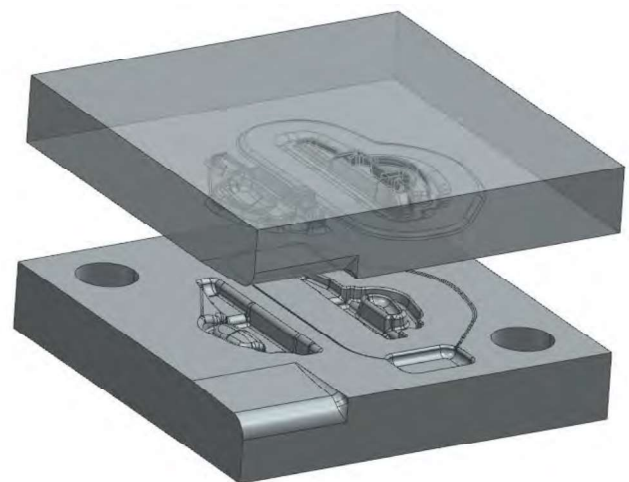
Figure 1. Upper and lower die for forging
