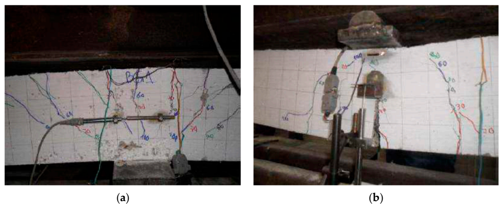
Figure 24. Experimental G1 beam failure: (a) mid-support section; (b) mid-span section.
