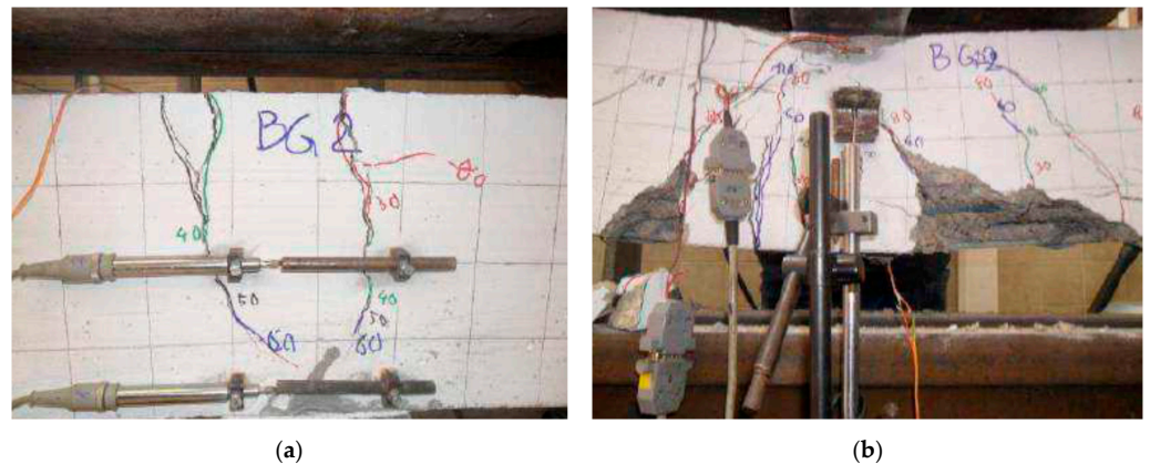
Figure 28. Experimental G2 beam failure: (a) mid-support section; (b) mid-span section.
