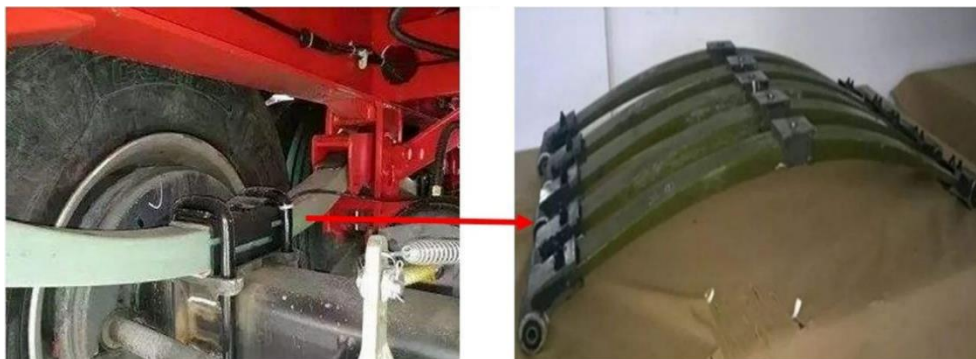
Figure 3 Location and typical construction of a GFRP composite leaf spring (Ma et al., 2021)
