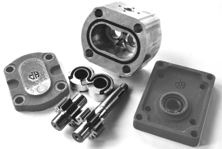
Figure 3. The analysed pump in disassembled representation
