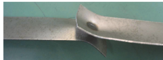
Figure 9 Deformed shape of welded joint obtained in experimental test
