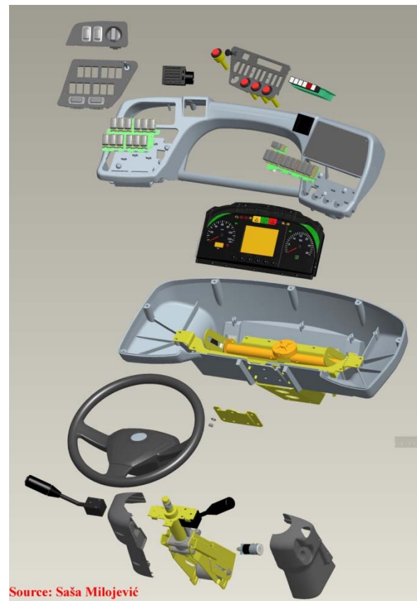
Figure 5. Internal design of podium dashboard for easy dismantling.
