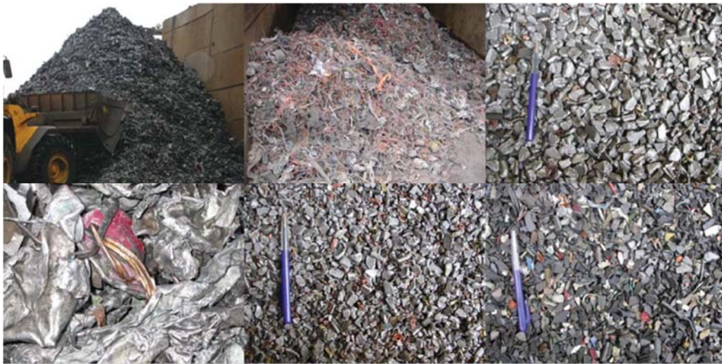
Figure 3. The diverse and distributed properties of recycling materials (clockwise: steel approximately 650 t. from 1,153 ELVs; copper fraction; Al/Mg/Cu/Zn fraction; plastic fraction; Al/Mg/Cu/Zn fraction; steel fraction).
