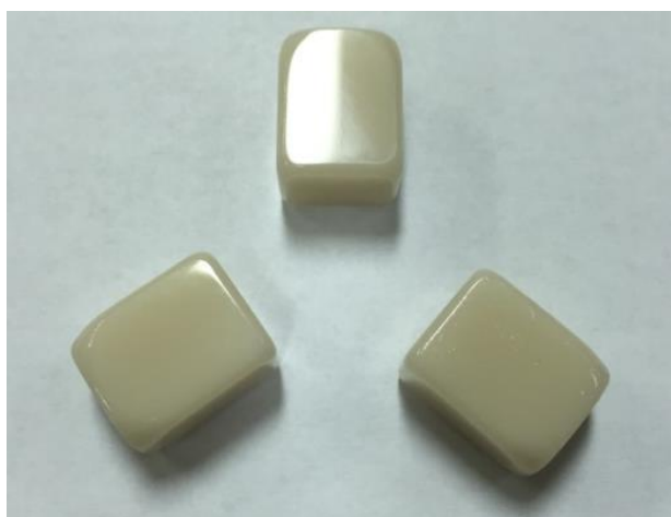
Fig. 2. Crystallized samples of lithium disilicate IPS e.max CAD, prepared with 3 different finishing procedures.
