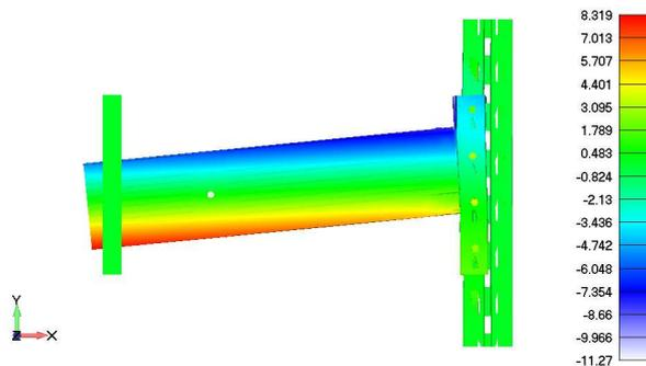
**Figure 12.** Filed of displacement in the  $x$  direction of the joint S80M-R140L.
