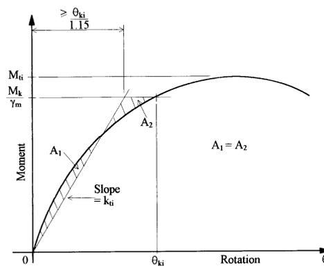
**Figure 7.** Derivation of connector stiffness.
