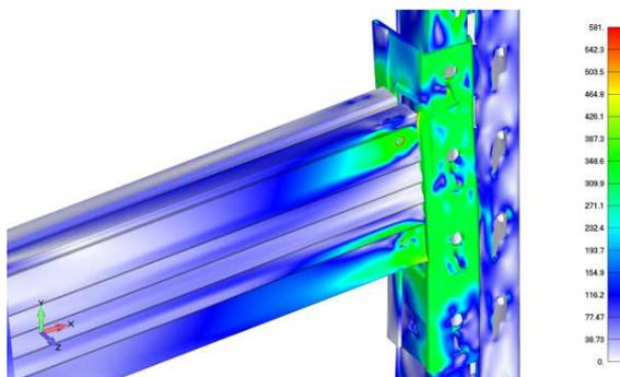
**Figure 14.** Field of equivalent stress for joint S80M-R140M.
