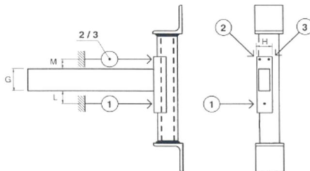
**Figure 6.** Devices for measuring displacement.
