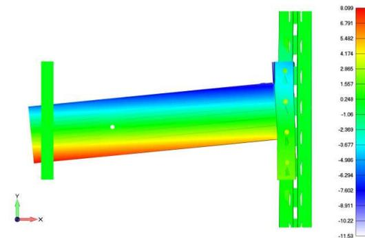
**Figure 13.** Filed of displacement in the  $x$  direction of the joint S80M-R140M.
