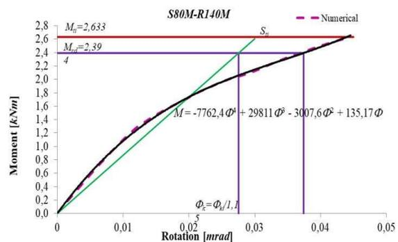
Figure 11. Moment-rotation curves for joint S80M-R140M.
