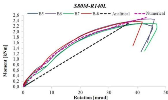
Figure 10. Moment-rotation curves for joint S80M-R140L.
