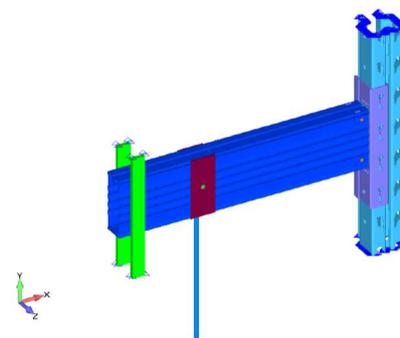
Figure 9. Boundary conditions and load.
