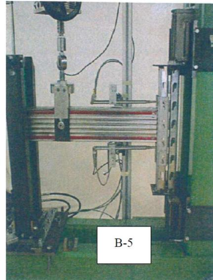
**Figure 3.** Arrangement for beam-end connector bending test. **Figure 4.** Photos of experiment settings.
