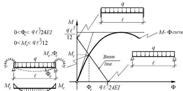
**Figure 2.**  $M-\Phi$  curve with structural properties and joint rotation.
