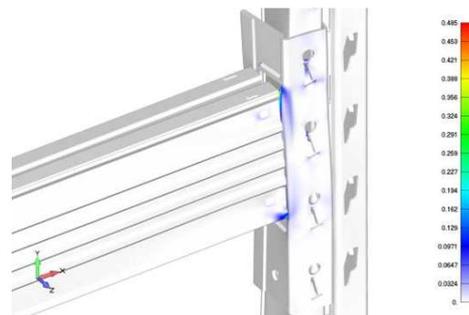
**Figure 15.** Field of equivalent plastic deformation for joint S80M-R140M.
