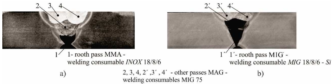
Figure 2. Microphotography of metallurgical samples of welded joints.
