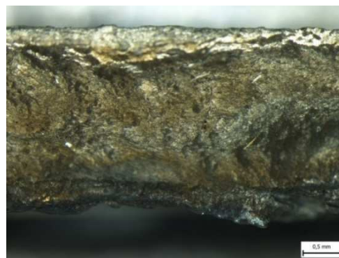
Figure 4. The cut edge surface of sample # 1 after the corrosion test.
