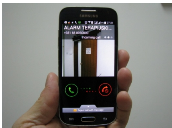
Figure 4. A call in progress on the responsible on call physician's mobile phone after the alarm system has been triggered
