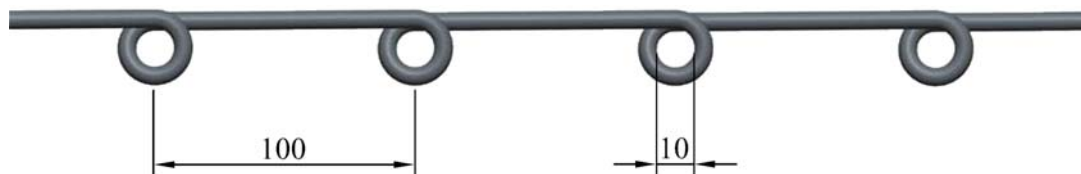
Fig. 1: The wire profile after the bending operation.
