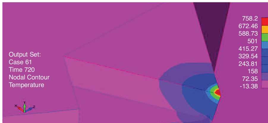
Figure 13. Temperature values within the tool with thermoelectric cooling located on the main back surface for T_h = 30\text{ }^\circ\text{C} and U = 23.9\text{ V} , after 12 minute
