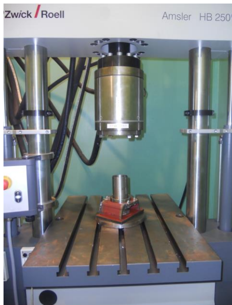
Figure 2 Servo-hydraulic machine ZWICK ROELL HB250
