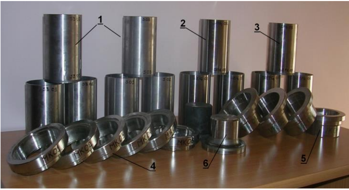
Figure 3 Samples: (1-Seamless tube without grooves, 2-Seamless tube with grooves length of 10 mm, 3-Seamless tube with grooves length of 110 mm, 4-Smaller cone angle bushing, 5-Larger cone angle bushing and 6-Splitting tool)
