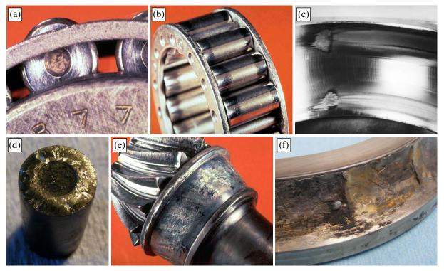
**Figure 2.** Bearing surfaces damaged by adhesive wear: (a) and (b) wiping of rollers (mild adhesive wear), (c) smearing of outer ring and (d), (e) and (f) change of colour and surface softening and flow of roller and inner rings material (severe adhesive wear).
