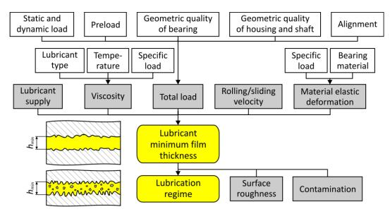
Figure 8. Parameters related to the lubricant film thickness and lubrication regime in a rolling bearing.
