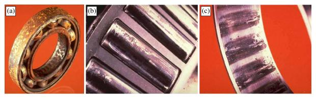
**Figure 7.** Bearing surfaces damaged by corrosive wear: (a) corrosion pits and rust all over the bearing and (b) and (c) discolouration of contact areas on rollers and outer ring.
