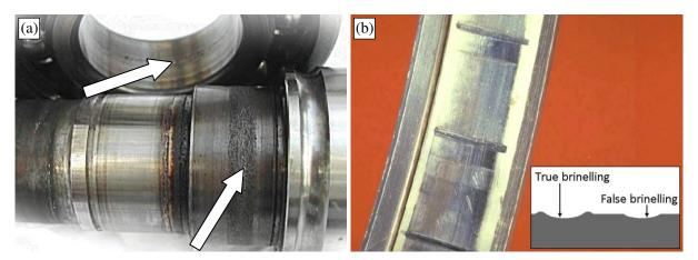
**Figure 6.** Bearing surfaces damaged by fretting (vibration) wear: (a) powder wear debris and change of colour on inner ring and shaft, due to the insufficient clearance and (b) equally spaced depressions and shiny worn areas (false brinelling) on inner ring due to the insufficient press fit.
