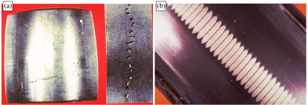
**Figure 5.** Bearing surfaces damaged by erosive wear (electrical erosion): (a) small craters (pits) on roller and inner ring due to the excessive voltage (electrical pitting) and (b) shallow and equally spaced groves (flutes) due to the current leakage (electrical fluting or washboarding).
