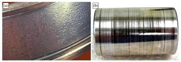
**Figure 1.** Bearing surfaces damaged by abrasive wear: (a) dull surface and visible dents (craters) on inner ring and (b) scratching and pronounced grooves on rollers.
