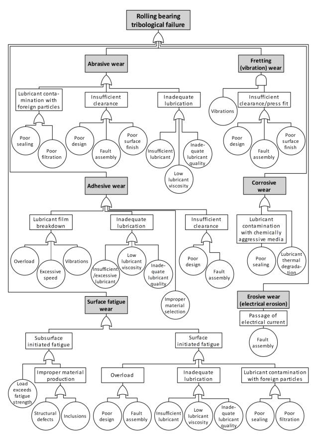
Figure 9. Fault tree of tribological rolling bearing failure.
